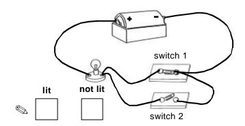
(b) Switch 1 is opened again, and switch 2 is closed. Tick one box (✓) to show if the bulb is lit or not now.
